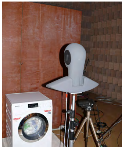
Fig. 6 Measurement of psychoacoustic product properties in anechoic chamber
