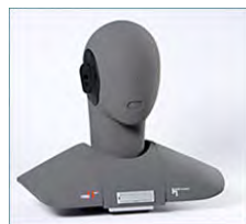
Fig. 3 Binaural measurement system – artificial head [8]
