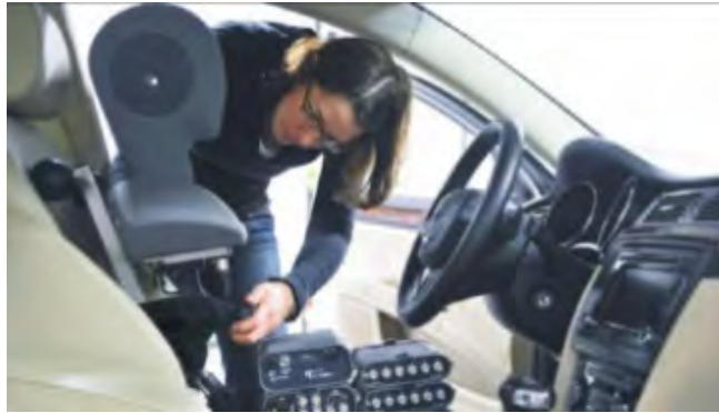
Fig. 5 Application of artificial head in the car interior [8]
