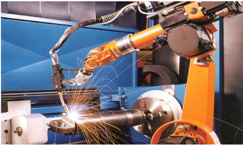
Fig 4. Welding – typical application of multirobotic systems
