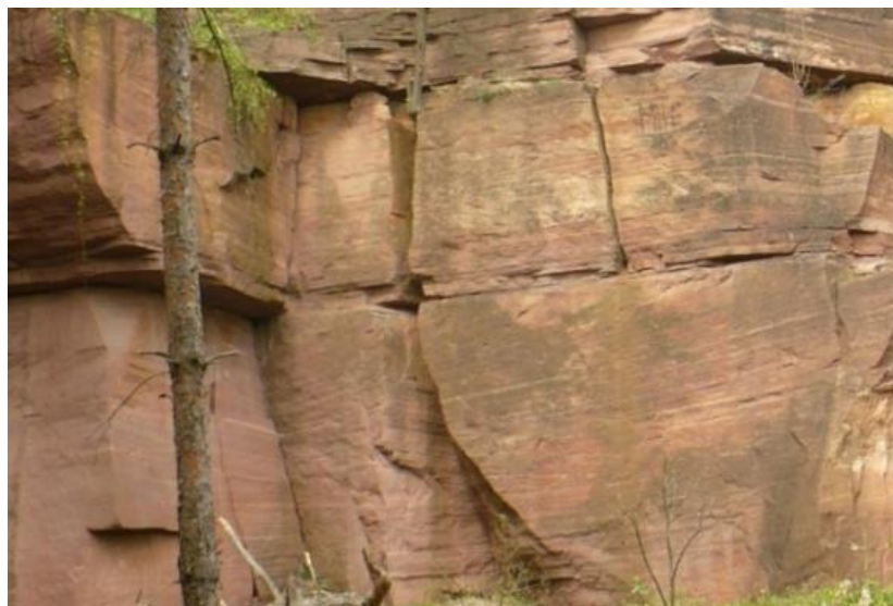
Fig.11 Jointing within Ciosowa quarry's sandstones (own elaboration)
