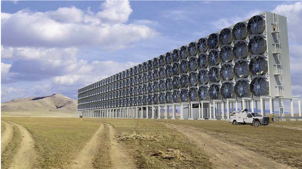
Fig. 3. A rendering of Carbon Engineering's air contactor
