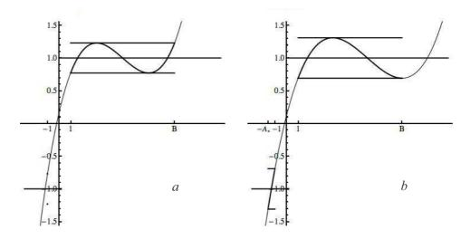
Fig. 1. Best polynomial approximation of sgn(x) with B = 10, n = 3. Solution on  $\{-1\} \cup [1, B]$  (a). Maximal extension with Chebyshev polynomials (b).
