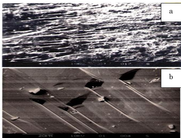
Fig. 7 – (a) As grown Etch pit are seen on the growth faces (b). The growth layers from the etch pits (black patches on the photograph)
