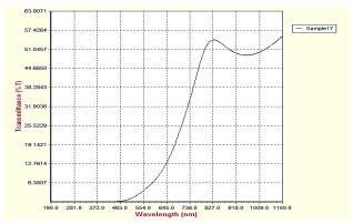
Fig. 2 - Transmittance vs. wavelength (200 °C and 3 hours)
