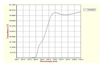
Fig. 4 – Transmittance vs. wavelength (300  $^{\circ}C$  and 3 hours)
