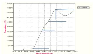
Fig. 1 – Transmittance vs. wavelength (200  $^{\circ}C$  and 2 hours)
