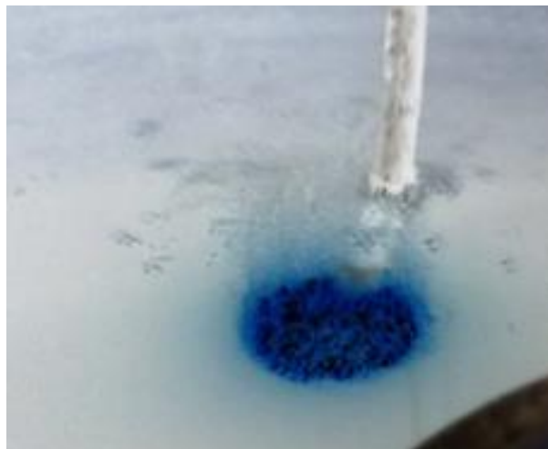
Fig. 1 – The process of anode-cathode oxidation in the mode of micro-arc discharges
