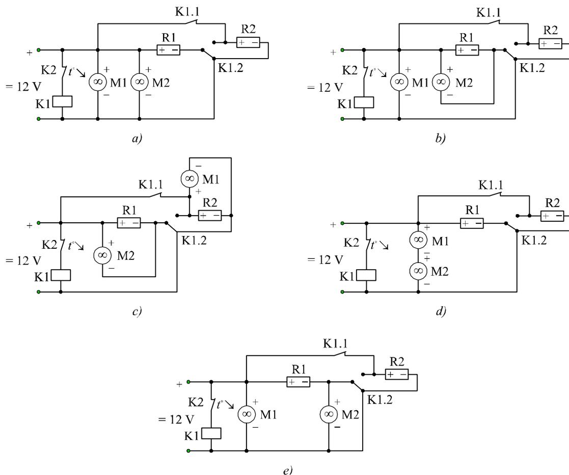
Fig. 3. Selected variants of electrical supply circuits of cooling unit of refrigerator under test.
