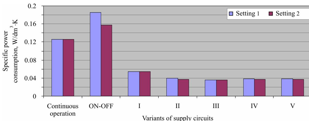
Fig. 7. Comparison of refrigerator specific power consumption for the investigated variants of supply circuits.
