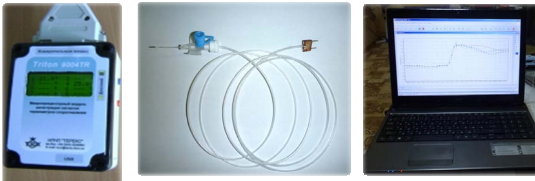
Fig. 1. Outside view of thermoelectric device for measurement of intraocular temperature.
