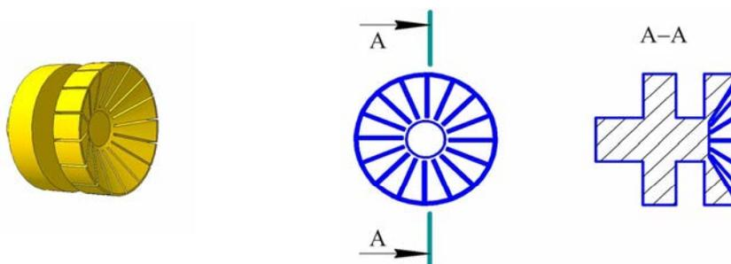
Fig. 5. Appearance and design of current leads.
