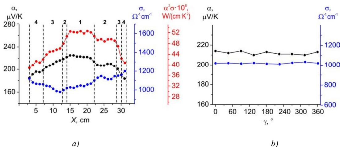
Fig. 10. Distributions of the Seebeck coefficient and electric conductivity in the n-type thermoelectric material based on  $\text{Bi}_2\text{Te}_3 - \text{Sb}_2\text{Te}_3$ , solid solution prepared by vertical zone melting method (a – along the length  $X$  of the rod, b – along the angle of rotation  $\gamma$  of the rod).
