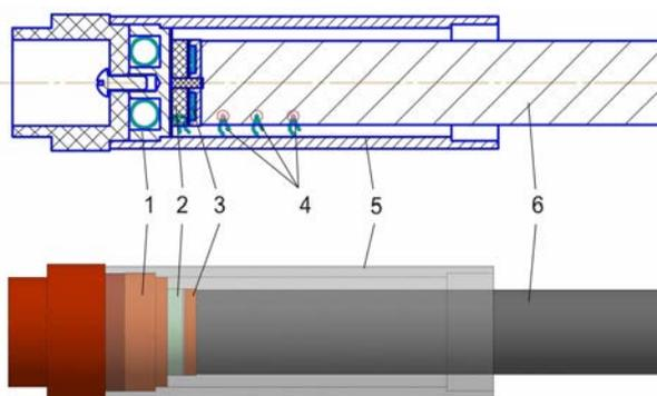
Fig. 8. Design of device for measuring thermal conductivity.
