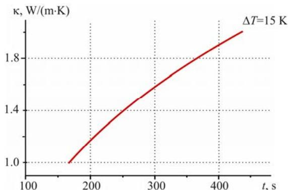
Fig. 9. Calibration dependence for determination of thermal conductivity.
