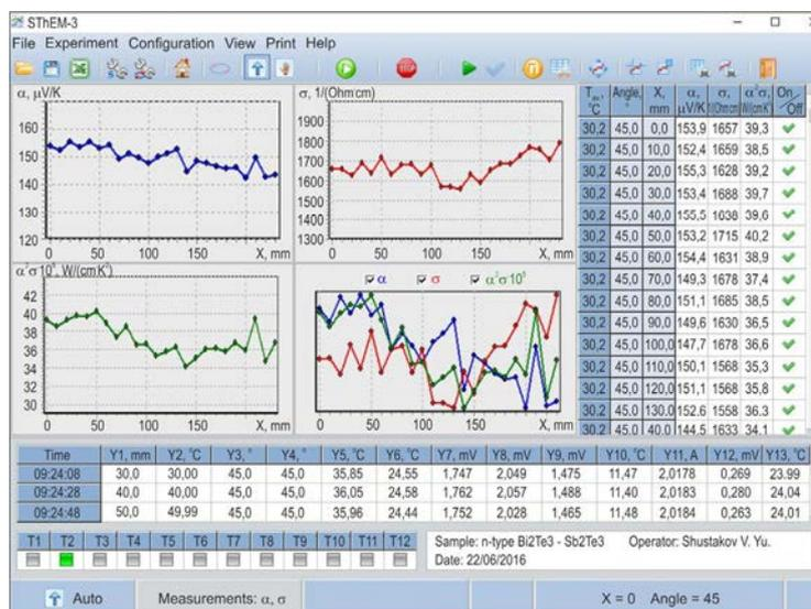
Fig. 7. Main window of measurement control program "SThEM-3".
