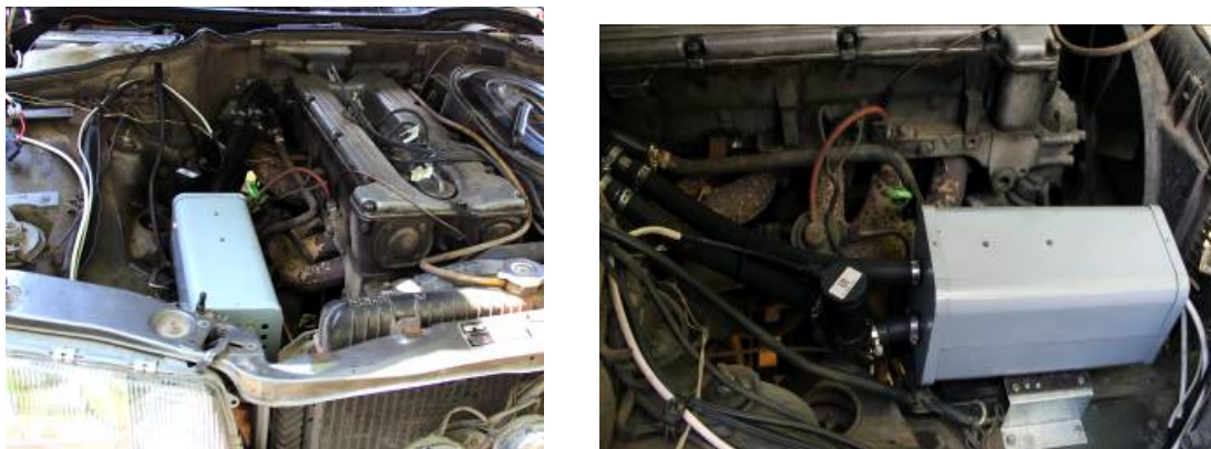
Fig. 8. Thermoelectric starting preheater in the “Mercedes” automobile.
