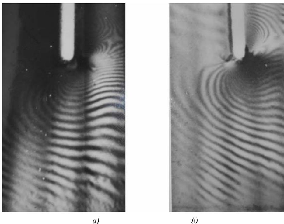
Fig. 1. Moiré pattern of analyzing crystal cut, reflection ( $\bar{2}20$ ): a) before etching; b) after etching  $\times 12$ .
