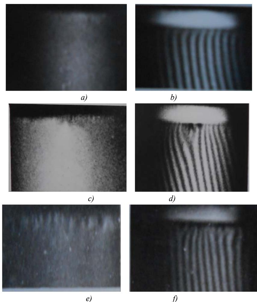
*Fig. 5. Topographic and moire images of the damaged layer depth. Reflection  $(\bar{2}20)$  a) b) surface machine processing  $(11\bar{2})$  with M5 powder; c) d) with M10 powder; e) f) with M28 powder  $\times 12$ .*
