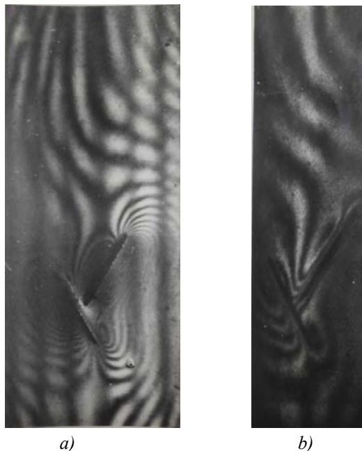
Fig. 9. Image of scratches applied at an angle to diffraction vector g_{220}^- : a) at room temperature; b) after annealing at 1023 K, \times 10 .
