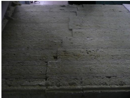
Fig. 17. Lamellas of insulation from which the specimens were cut
