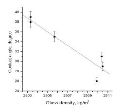
**Fig.** Contact angle as a function of density
