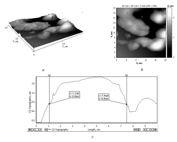
**Fig. 2.** 3D- (*a*) and 2D (*b*) maps of the surface and cross sections profile (*c*) between markers 1 and 2 for mixed oxide system Al | Al<sub>2</sub>O<sub>3</sub>·CoO<sub>x</sub> with cobalt content 8.7 at. %. Scanning area 20×20 μm
