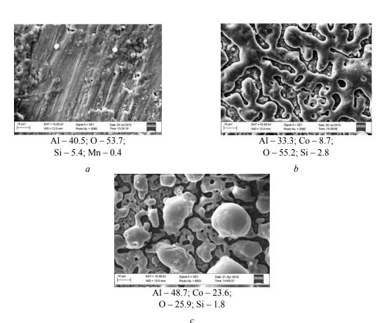
**Fig. 1.** Surface morphology and composition (at. %) of PEO coatings on AL25:  $a - Al | Al_2O_3$  obtained in electrolyte 200 g/l K<sub>4</sub>P<sub>2</sub>O<sub>7</sub> with current density  $i_1=8 \text{ A/dm}^2$ ; mixed oxide systems Al | Al<sub>2</sub>O<sub>3</sub>·CoO<sub>x</sub> obtained in PEO two stage modes ( $i_1=8 \text{ A/dm}^2$ ,  $i_2=2.5 \text{ A/dm}^2$ ) in diphosphate electrolyte with addition of CoSO<sub>4</sub> of concentration, g/l: b - 10; c - 30. Magnification 1000
