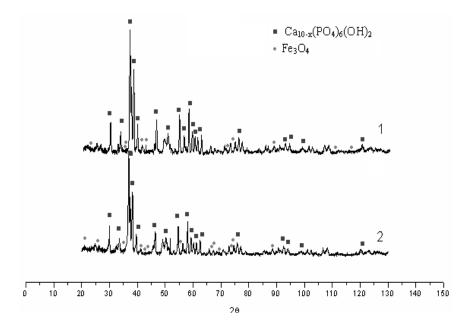
**Fig. 1.** Diffractograms of studied powder materials: *1* – BHA + Fe<sub>3</sub>O<sub>4</sub> (chem. method); *2* – BHA + Fe<sub>3</sub>O<sub>4</sub> (phys.-mech. method)
