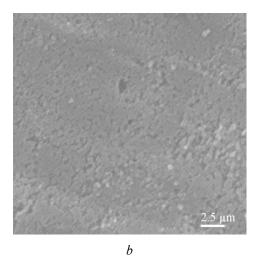
**Fig. 2.** Microstructure of studied materials (×5000):  $a - BHA + Fe_3O_4$  (phys.-mech. method);  $b - BHA + Fe_3O_4$  (chem. method)
