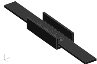
Figure 1. Full geometric model of the test sample for fatigue characteristics of the bolted connection with PCM
