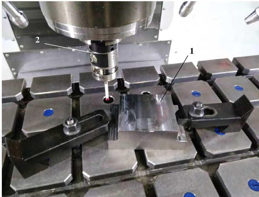
Fig. 4. Measurement of workpiece control points
