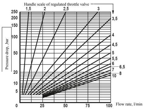
Fig. 2. Characteristic  $\Delta p$  - qv (Pressure drop – Flow rate) of regulated throttle valve NG16 type
