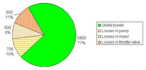
Fig. 4. Energy balance of power in first version of operation
