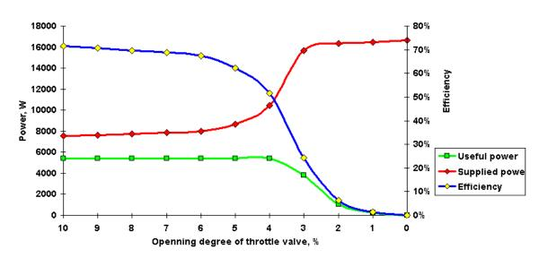
Fig. 14. Diagram of energy balance by different opening degree of throttle valve
