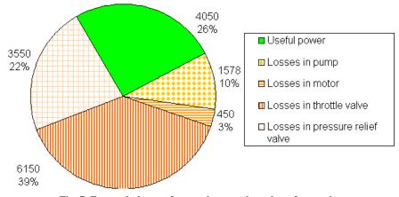
Fig. 7. Energy balance of power in second version of operation
