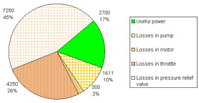
Fig. 9. Energy balance of power in third version of operation
