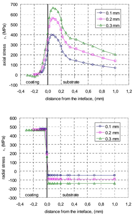
Fig. 3. Axial ( $s_y$ ) and radial ( $s_x$ ) stress profiles across the coating thickness calculated in the Ti/AlN system for three coating thicknesses (left- along line 1, right - along line 2 in fig. 2)
