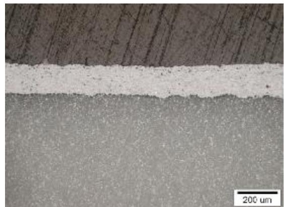
Fig. 4. The microstructure of titanium coating deposited onto the AlN substrate by the D-gun technique ( $r100$ )
