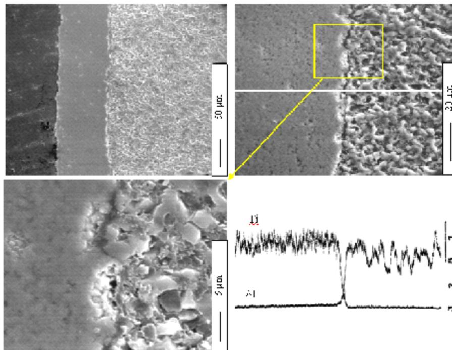
Fig. 5. The microstructure of titanium coating deposited onto the AlN substrate by the D-gun technique with linear distribution of Ti and Al elements
