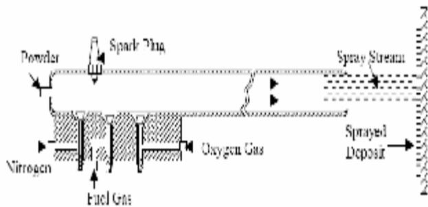
Fig. 1. The scheme of D-GUN thermal spraying method [2]
