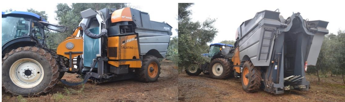
Fig. 1. Towed olive harvester CV5045 built by Pellenc
