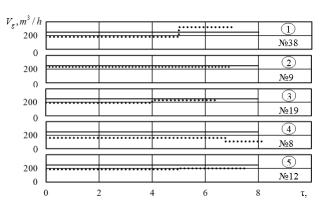
Figure 6. Changes in the supply of natural gas  $(V_g)$  during the ladles heating when fuel burning pulsating resonance
