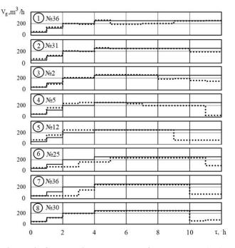
Figure 4. Changes in the supply of natural gas  $(V_g)$  during the ladles drying when fuel burning pulsating resonance
