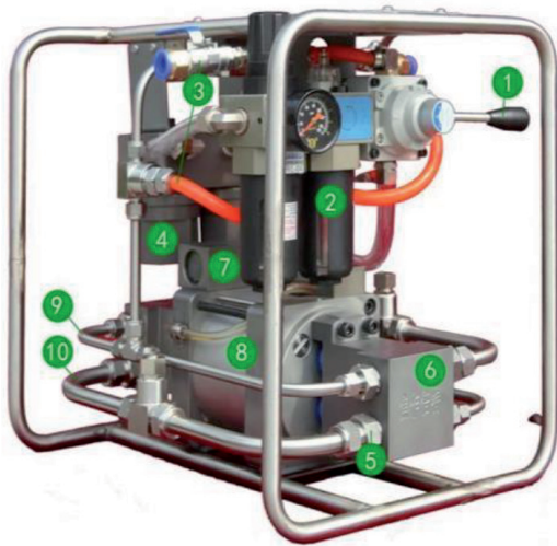
Figure: 1 Station control switch 2 Air triplets 3 Gas pipeline 4 Air purifier 5 One-way valve 6 Slurry cylinder 7 Stroke switch 8 Pneumatic master cylinder 9 Slurry draining pipeline 10 Slurry extracting pipeline
