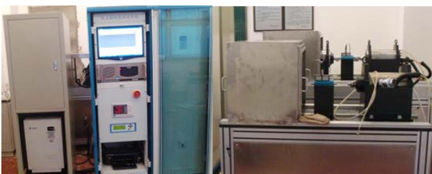
Figure 10. Integrated performance test platform of ceramic spindle
