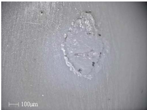
Figure 2. Fatigue spalling of ceramic race
