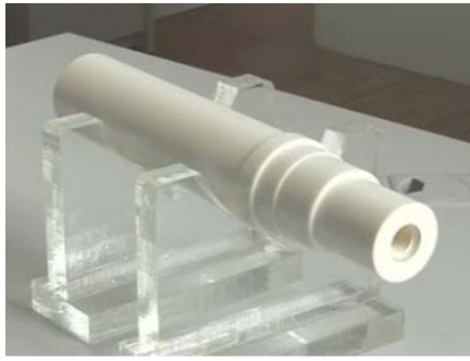
Figure 6. Full-ceramic motorized spindle of full-ceramic shaft
