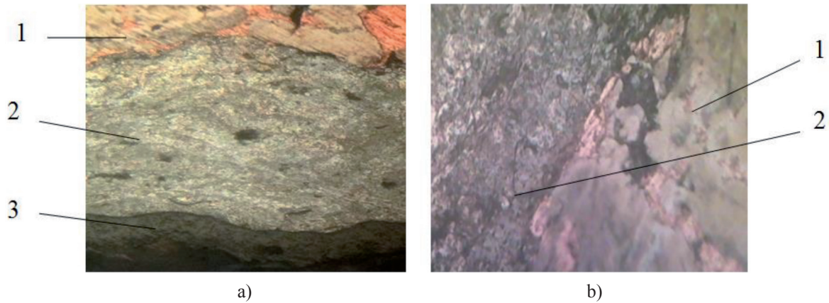
Figure 9. Microstructure non-pickled areas of the sample at magnification: a) \times 100 ; b) \times 250 1 - base metal; 2 - electro metallic coating; 3 - plasma electrolytic oxidized coating
