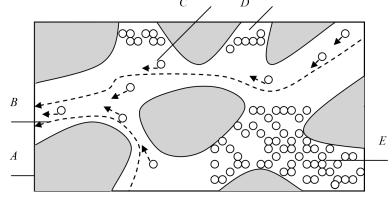
Figure 1. The scheme of the filtration efficiency of the porous permeable materials of saponite - titanium system composite: A - porous permeable medium; B - water movement; C - particles release; D - water associated with the precipitate; E – precipitate
