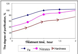
**Figure 3.** Influence of high-frequency electric treatment on the degree of water purification
