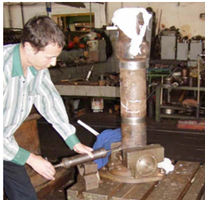
Figure 4. Stages of restoration of hydraulic cylinder
