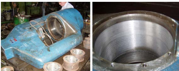
Figure 4. Stages of restoration of hydraulic cylinder
