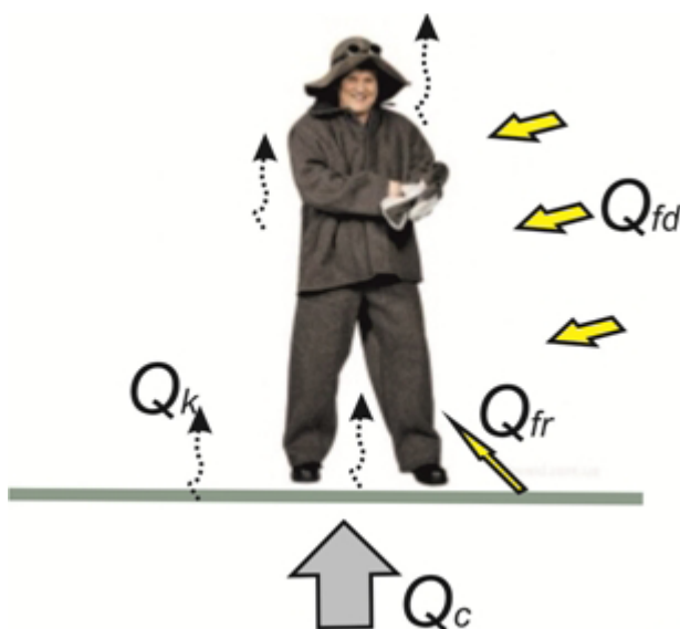
Figure 3. Diagram of impact of external thermal streams: direct and reflected beam ( Q_{fd} and Q_{fr} ) respectively; convective ( Q_k ); conductive ( Q_c ) on the metallurgist
