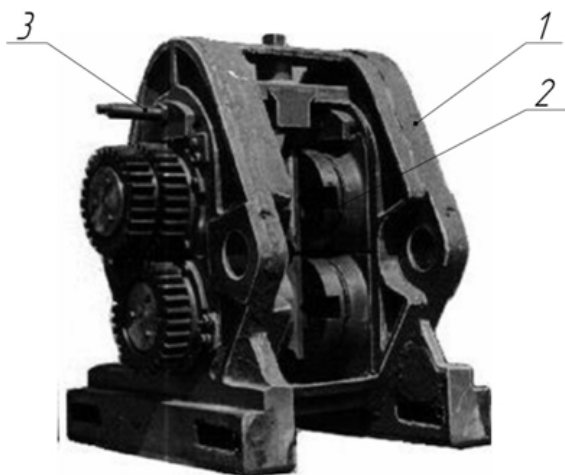
Figure 1. Working stand cold rolling mill pipe of rational design
