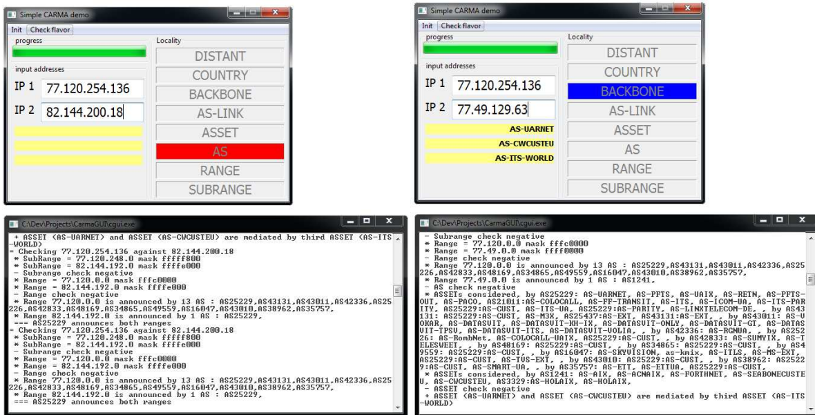
Figure 2 – CARMA demo interface featuring two IP addresses with calculated locality class of “AS” and “backbone” respectively
