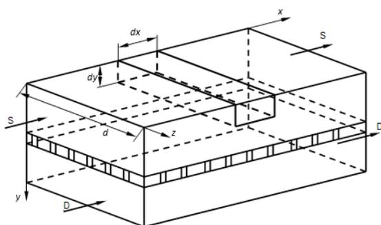
Fig. 1. The scheme of the elementary volume in the membrane module: S – solution, D – distillate
