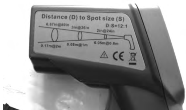
Fig. 16. Laser pyrometer, which was used for the study
