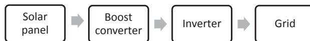
Fig. 1. Chain diagram of an offline electric power supply system based on solar batteries
