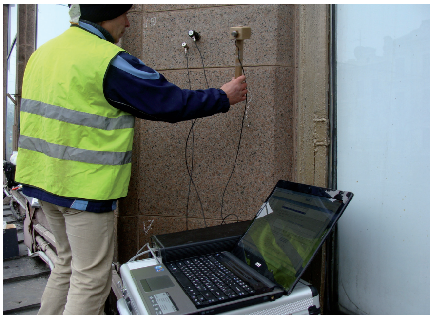
Fig. 2. Study of surfacing materials adhesion state using TKC-2 complex.
