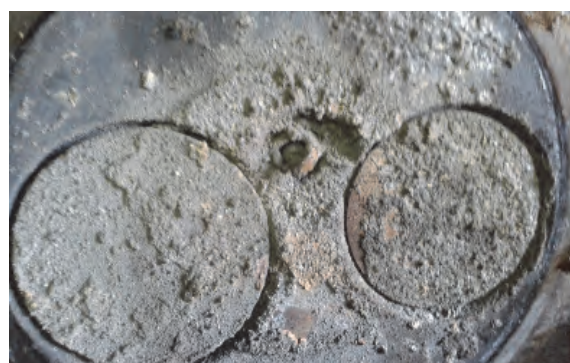
Fig. 6. Effects of direct use of crude biogas (no purification)
