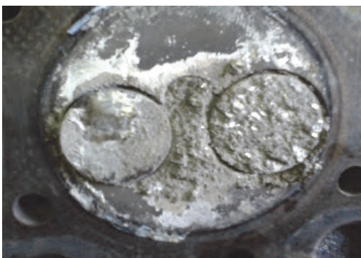
Fig. 6. Effects of direct use of crude biogas (no purification)
