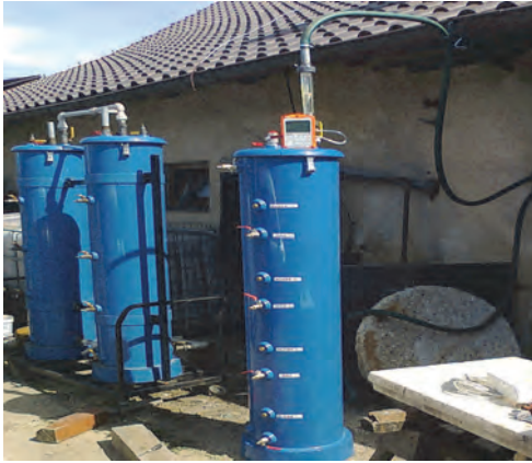
Fig. 3. Research stand in a small-scale agricultural biogas plant
