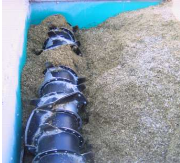
Fig. 3. Proportioner of fat-containing biomass into anaerobic fermentation chamber (photo: Jan Cebula)
