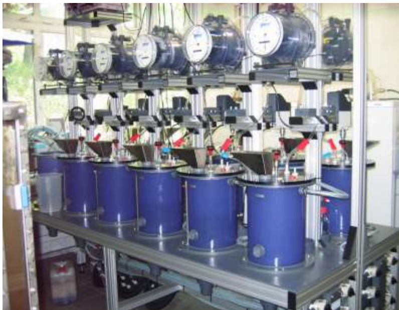
Fig. 6. The reactors for the research of anaerobic fermentation course during fat wastes processing (photo: Jan Cebula)
