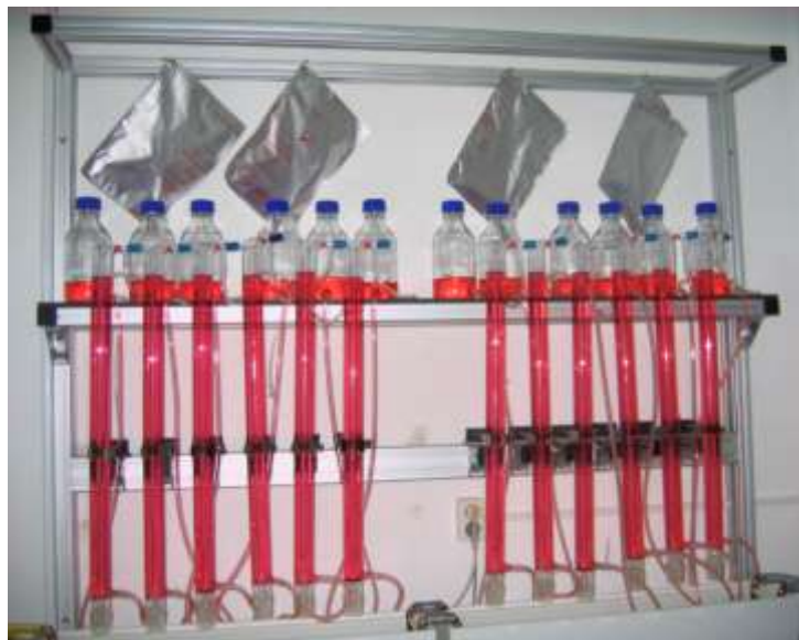
Fig. 5. The laboratory-scale system for measurement of biogas generation potential of fat wastes and appropriate process kinetics (photo: Jan Cebula)
