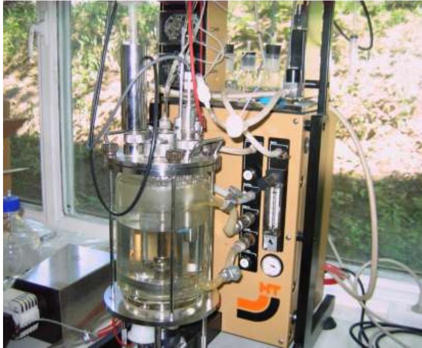
Fig. 7. Laboratory bioactor for the measurement of methane fermentation process course(photo: Jan Cebula)
