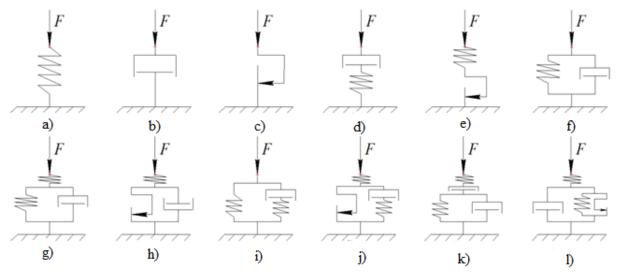
Fig. 1. The main rheological models, where F – external force: a – Hooke; b – Newton; c – Saint-Wenan; d – Maxwell; e – Prandl; f – Voigt; g – Kelvin; h – Binham; i – Poynting-Thomson; j – Shvedov; k – Burgers; I – Imlinskiy.
