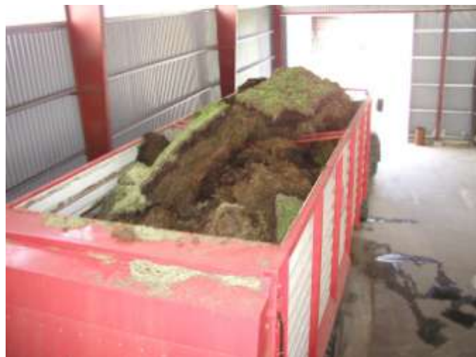
Fig. 4. The self-unloading trailer used for transportation of silage in a biogas plant (photo J. Cebula)
