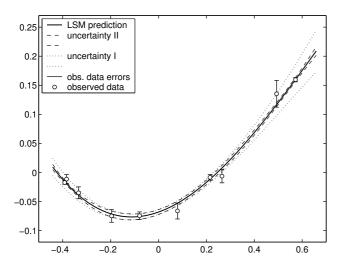
Figure 1: The illustrative figure displays the time dependence of an observed quantity measured with the accuracy denoted by the abscissa. The continuous line represents LSM fit by the polynomial of the 3-rd order (cubic parabola). Expected uncertainties of this prediction calculated by the formula Eq. 16 are denoted by dotted lines, true uncertainties given by Eq. 17 are signed by dashed lines.
