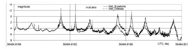
Figure 2: Simultaneous measurements of the satellite brightness from two UMOS observation points. The data received on July 11, 2013 in Odessa and Yevpatoria. Vertical lines correspond to the satellite's rotation period.
