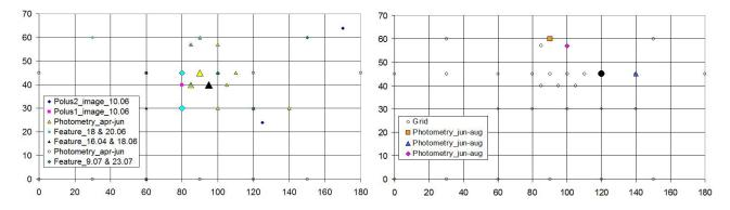
Figure 4: The optimal solution for the EnviSat satellite rotation pole obtained with various techniques for the period from: a) May to June 2013; b) June to August 2013.
