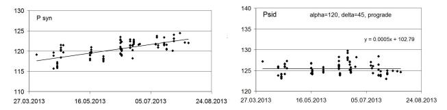
Figure 3: a) the measured values of the EnviSat space craft synodic rotation period; b) the optimal solution for the rotation pole ( $\alpha_p = 120^\circ$ ,  $\delta_p = 45^\circ$ , the prograde rotation), deduced by the method accounting for parallactic shift of flashes on the light curve. At that, the average sidereal rotation period within 4 months is almost constant and equals to 125.6 sec.
