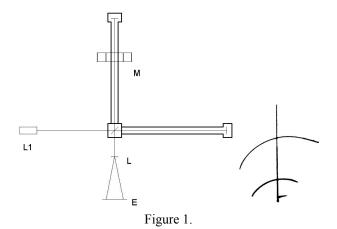
Legend elements: L1- laser, E – screen, L – focusing lens, M – a rotating disk. The length of the shoulder is 87 cm. Hard
