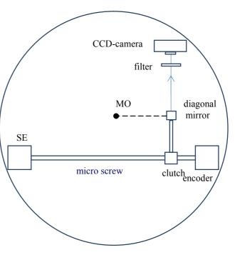
Figure 2: Optical-mechanical scheme of photometer second channel
