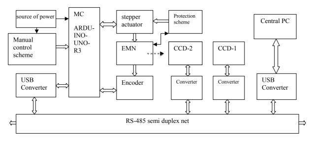
Figure 3: Structure of two-matrix photometer control system structure
