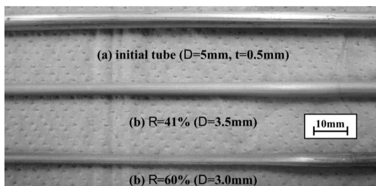
Fig. 5. Photograph of deformed tubes after dieless drawing process in a single-pass under a condition of heating temperature of 450°C.
