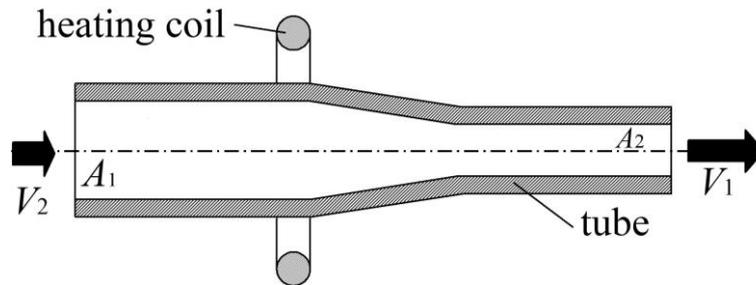
Fig. 1. Schematic illustration of dieless drawing process
