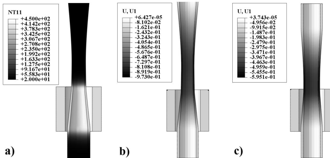
Fig. 2. Results of numerical simulation at the cross section of pipe for length of heating element equal to 10 mm: a) distribution of temperature for  $R = 60\%$ , b) distribution of displacement for  $R = 60\%$ , c) distribution of displacements for  $R = 41\%$
