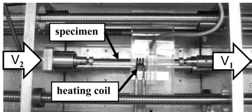
Fig. 4. Photo of the experimental setup of dieless drawing process.
