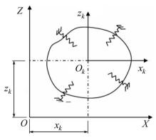
Fig. 4. The linear displacement, with original stiffness center in mind  $O_k$
