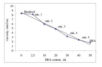
Fig. 3. The dynamic viscosity of the investigated mixtures under standard conditions
