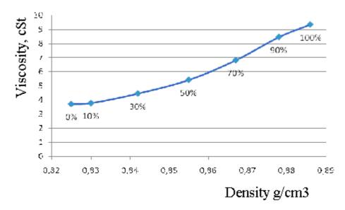
Fig. 10. Relationship between viscosity and density for the mixtures of DF with MERO at different ratios
