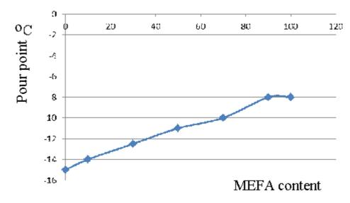
Fig. 9. Temperature of freezing of MERO mixtures with DF at different content of MERO (0, 10, 30, 50, 70, 90, 100 % )
