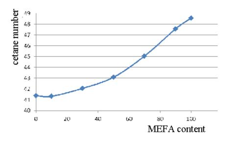
Fig. 8. Growth of cetane number at increase of content of biodiesel in a fuel mixture
