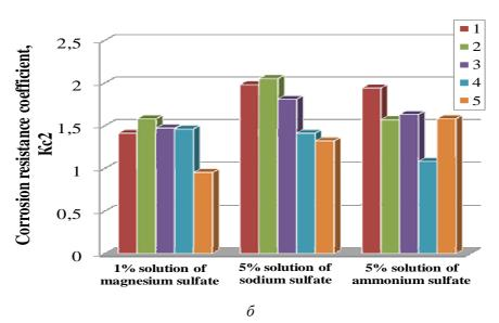
**Fig. 2.** Variation of corrosion resistance coefficients  $K_{C1}(a)$  and  $K_{C2}(b)$  for coating compositions: "portland cement + granulated slag + natural zeolite + salts electrolytes" (1); "portland cement + granulated slag + salts electrolytes" (2); "portland cement + granulated slag + natural zeolite + salts electrolytes + GKJ 136-41 (3); Penetron (4); uncoated control sample (5) (after 126 days the test)
