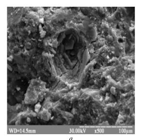
with optimal component  $Na_2CO_3$ :  $Na_2SO_4$ :  $NaNO_3 = 4:5:1$ , is represented mainly by hydrosilicates of calcium and a hydrosulphoaluminate type of ettringite structure (AFt that AFm), that occlude its pore space both reducing water absorption and water penetration in time.
