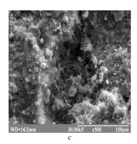
Fig. 1. SEM micrograph of the sample, after 1 year of hardening, based on Portland cement with the addition of granulated blast furnace slag a with the following modification of natural zeolite b or complex supplement containing natural zeolite and salt electrolytes c
