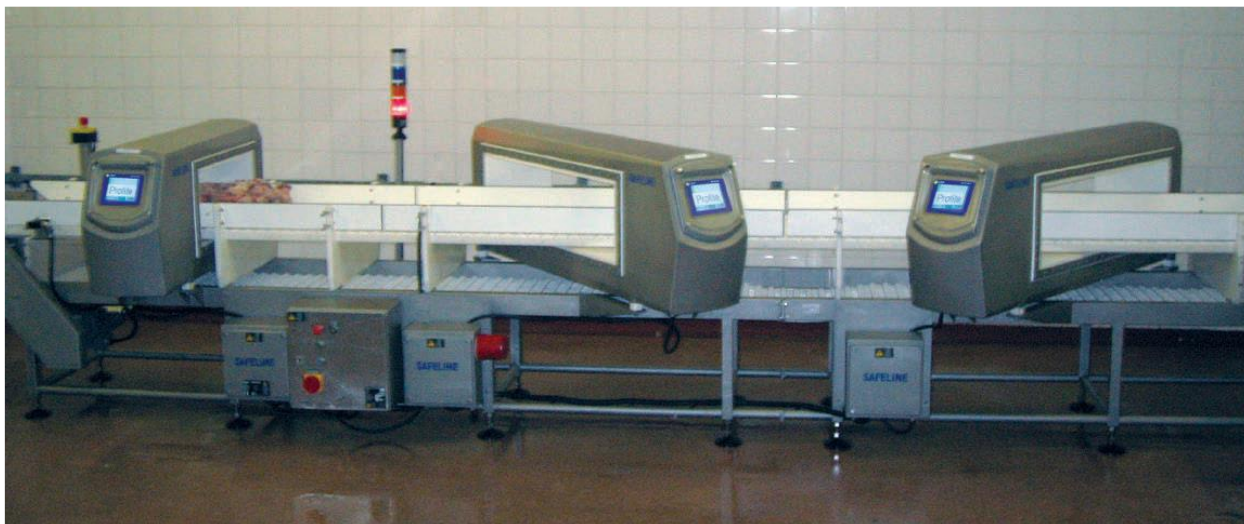
Fig. 5. SAFELINE Profile metal detector with three detection units is intended to survey meat portions up to 25 kg. Manufacturer - Mettler-Toledo Safeline (UK)
