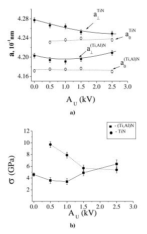
Fig. 2 – Influence of the amplitude of the pulsed bias potential on the characteristics of the stress state of TiN and  $\rm Ti_{0.5*}Al_{0.5}Y_xN$  coatings (on the results of X-ray tensometry): a - the period of the crystal lattice, and b - the level of residual stresses
