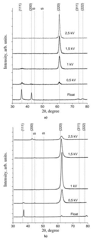
**Fig. 1** – X-ray diffraction patterns of vacuum-arc coatings deposited from the filtered plasma at different amplitude pulsed substrate bias potential (emission of Cu-K<sub>a</sub>, dashed lines show the position of peaks of TiN (PDF No 38-1420), "S" indicates the line of the substrate): **a** - coating TiN; **b** - coating Ti<sub>0.5-x</sub>Al<sub>0.5</sub>Y<sub>x</sub>N
